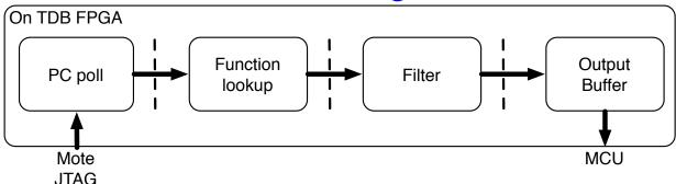
• The pipelined architecture enables us to keep up with the rate of the OCDM event stream
